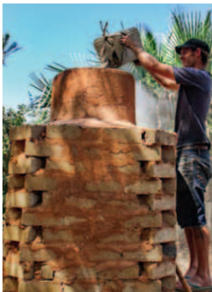
Anticlockwise from above: The temperature in the kiln was checked regularly with a sensor; recharging during the burn with the oyster shells/charcoal mix; insulation infill for the walls of the kiln; three successful firings produced a good supply of lime.
