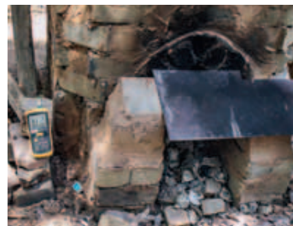
Anticlockwise from above: The temperature in the kiln was checked regularly with a sensor; recharging during the burn with the oyster shells/charcoal mix; insulation infill for the walls of the kiln; three successful firings produced a good supply of lime.
